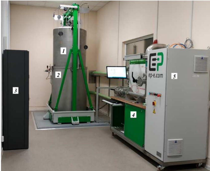
1 – bell (in highest position), 2 - oil tank, 3 - cabinet of climate precision system, 4 – test bench, 5 - cabinet of automated control system
